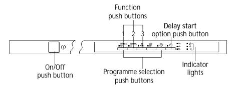
**Function push buttons:** in addition to the dishwashing programme selected, the following functions can also be set with the help of these buttons:
